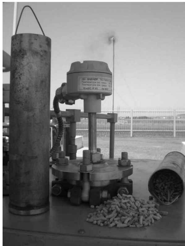
Fig. 3. Catalyst unit and pelletized catalyst.
